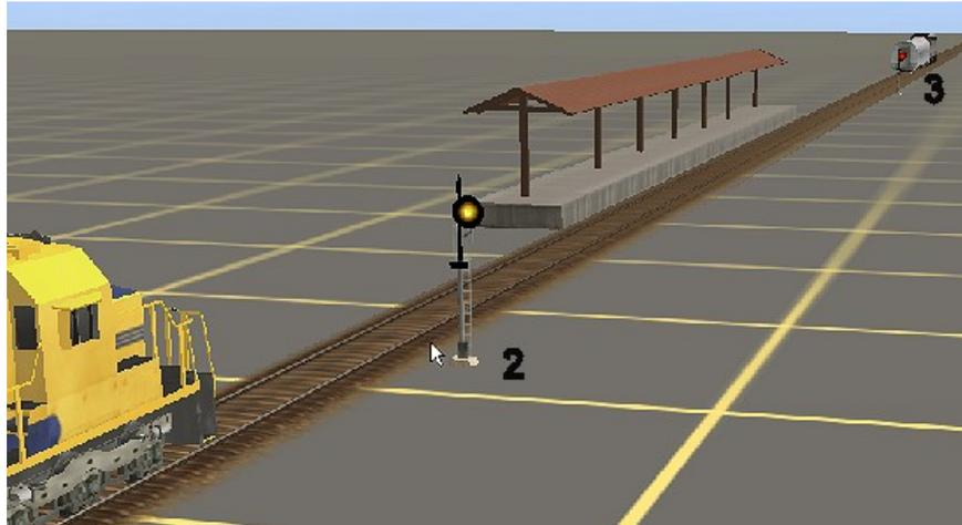
After the passenger train leaves the station block between signals 2 and 3, the AI will now see that block as clear. Accordingly, signal 2 will turn to yellow, allowing the freight train to proceed at restricted speed.
