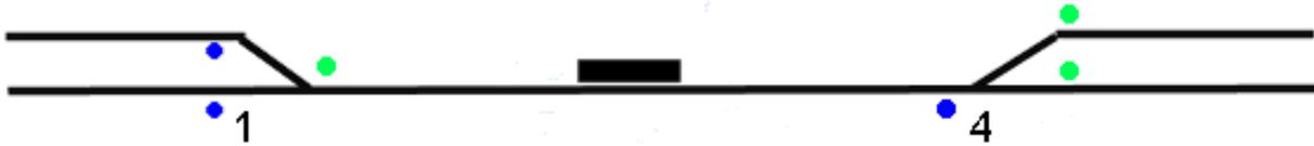
If you're new to Surveyor, I suggest you follow the design above. The blue dots at signal 1 and the green dots at 4 are all xx-04 signals. The green dot at 1 is an xx-02 and the blue dot at 4 is a xx-02L, since it's a left divergence. (Since this map is USA-based, the signals are placed to the right of the track.)
