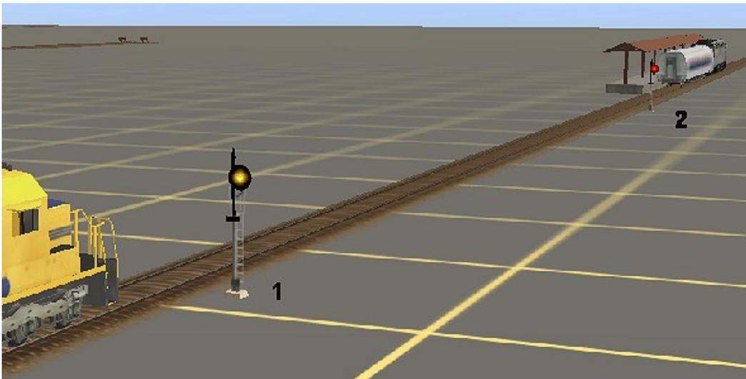
In the picture, we have a 60mph mainline track, with a freight train at signal 1 and a passenger train standing in the station on the other side of signal 2. The red signal is the “home” signal, protecting the rear of the passenger train. The yellow signal is called an “approach” signal, and it is designed to give advance warning to track conditions ahead.
