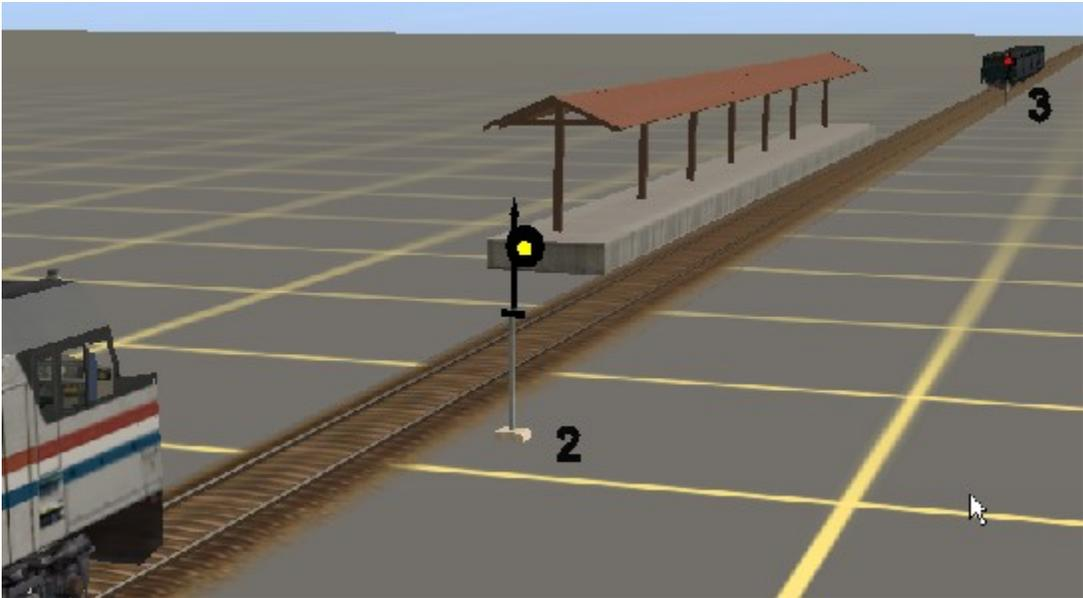
Now those of you pretty sharp with signals will have noticed that signal #2 is a USA-05, and as such it is a *permissive* signal, meaning that a train is permitted to pass red at restricted speed, provided it comes to a complete stop first on reaching the signal. Under these conditions, on a Trainz route a manual driver could pass the signal after stopping and then pull into the station. (AI-controlled trains, though, will not pass a permissive.)
