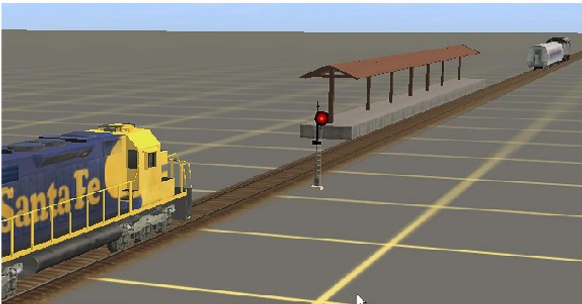
It stays red, because the passenger train is still occupying the block following the signal. In fact, the signal will continue to stay red until the passenger train completely passes the *next* signal, even if that signal is five miles down the track.
