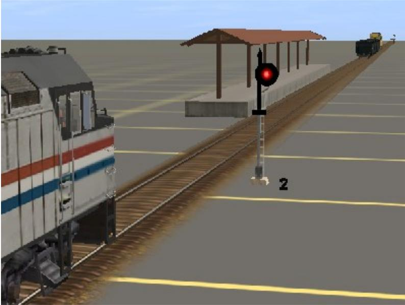
Notice that even with the freight train gone, the passenger train is still stuck by red signal number 2, even though the track into the station is obviously clear. Without signal number 3 on the other side of the station, the passenger train will be stuck at #2 signal, until the freight train clears signal #4, far down the track.
