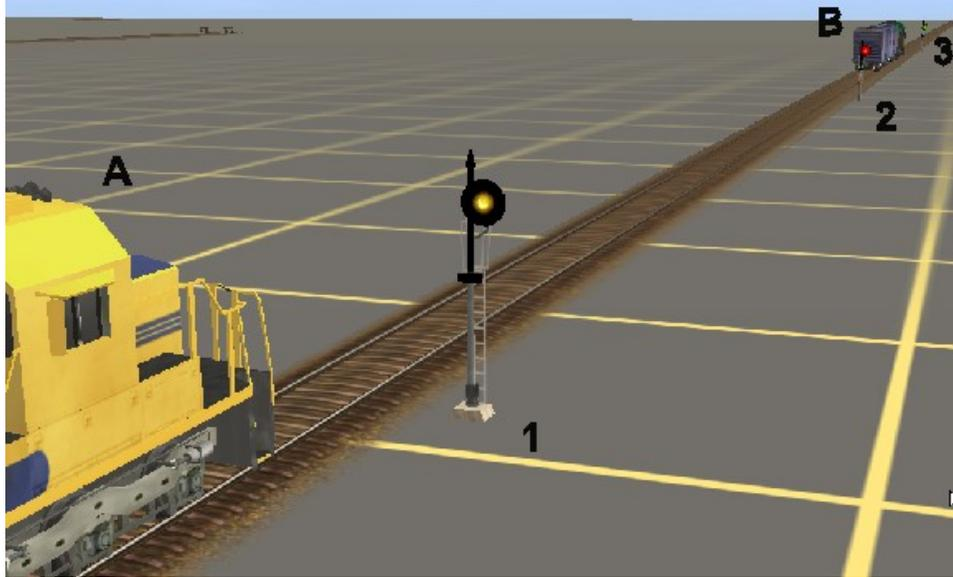
Let's say the distance between signals 1 and 2 is two miles. Because it's under restriction, train A must run the whole two miles at restricted speed, even if train B leaves the block between signals 2 and 3.
