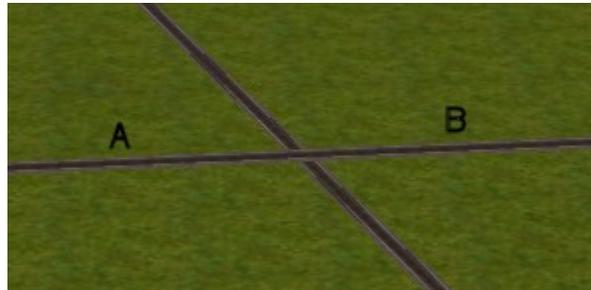
Insert new spline points at A and B above. Then type the height you want for your elevated track in the vertex tool window. I used fifteen for this example, but you can use any value you wish.
