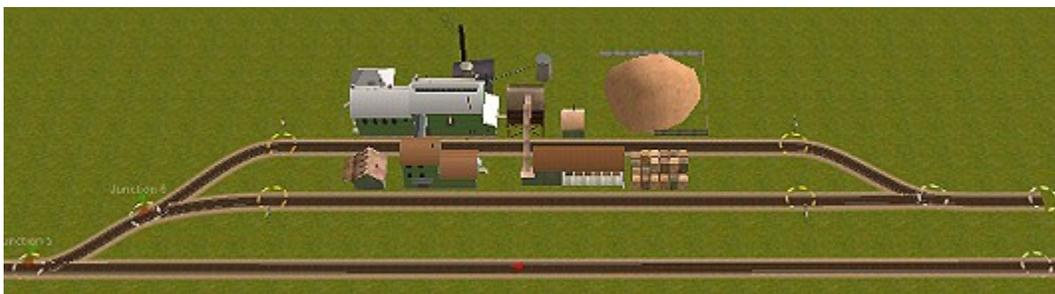
In the arrangement above, mainline trains that approach from the right have to back into the industry. Trains approaching from the left go in head-first, but can use the switch at the far right to 'run around' the train and couple to the rear if necessary to head back to the left. An alternate arrangement, if space and budget permit, is to provide a reverse loop to the right of the industry, like this:
