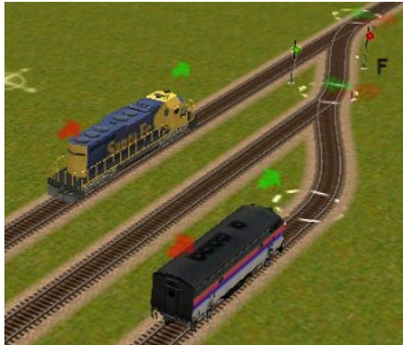
There's a problem with this arrangement, though. If the mainline switch is set for the SD40, as shown above, then the SD40 can advance past the signal and stop, ready to enter the industrial area. That part's okay. But placing the industry-area signal at F allows the F7 to advance to that signal, thereby blocking the SD40 from entering. Get the idea?
