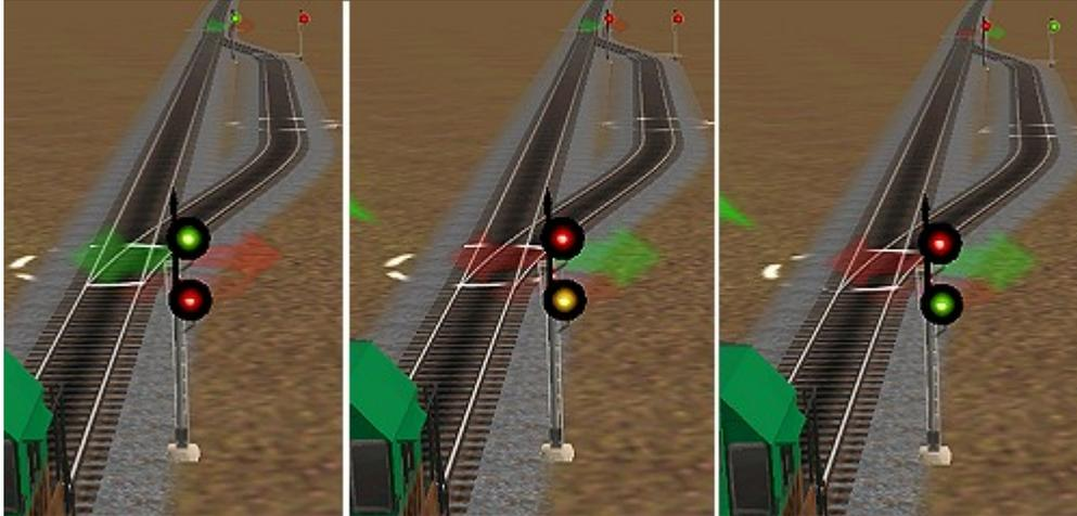
In the drawings below, we have the same indications for the USA 2 02 signal, also using USA 2 04's at the far end.
