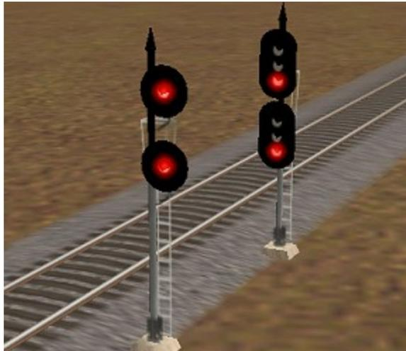
The signals above are USA 02 and USA 2 02. They probably have the same equivalents in other signal systems. In typical use, the upper head shows the aspect for the mainline and the lower head is for the diverging path.
