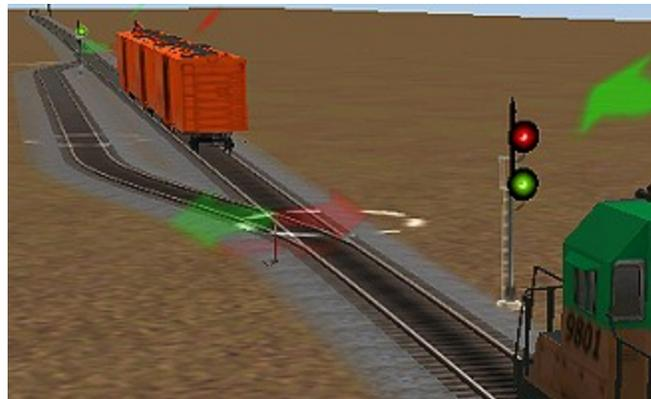
Even though the mainline is blocked by a string of boxcars, the train still has a clear path through the pass track, and the 'L02' shows a diverging path clear aspect.
