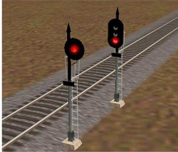
These two signals are USA 05 and USA 2 05. They look similar to the '04', except they have the nameplate halfway up the mast. These signals are permissive; after a stop, the driver can continue at restricted speed. As with the '04' signals, the '05' signals for other regions probably work in a similar manner.
