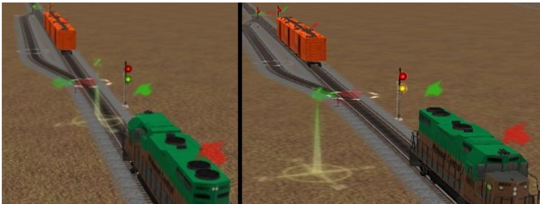
The two pictures above are of the same junction, but there is an important difference between them. In the left picture, the loco is facing *toward* the turnout. The signal indication is correct. In the right picture, the loco is facing *away* from the turnout. In this case, the signal is behind the locomotive instead of in front of it, and the signal indication is for a train moving away from the switch.
