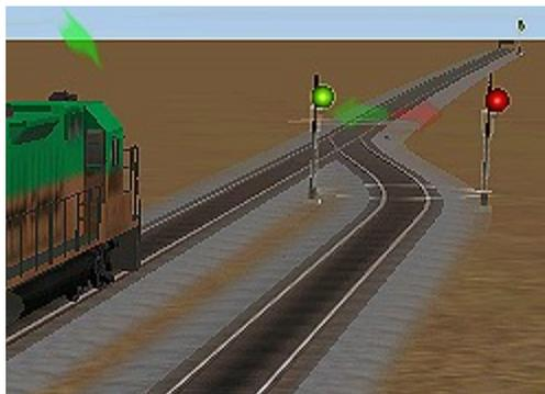
As you see in the drawing, it's critical that the train stop if the turnout is facing the wrong way, so we use an '04' or other absolute signal.
