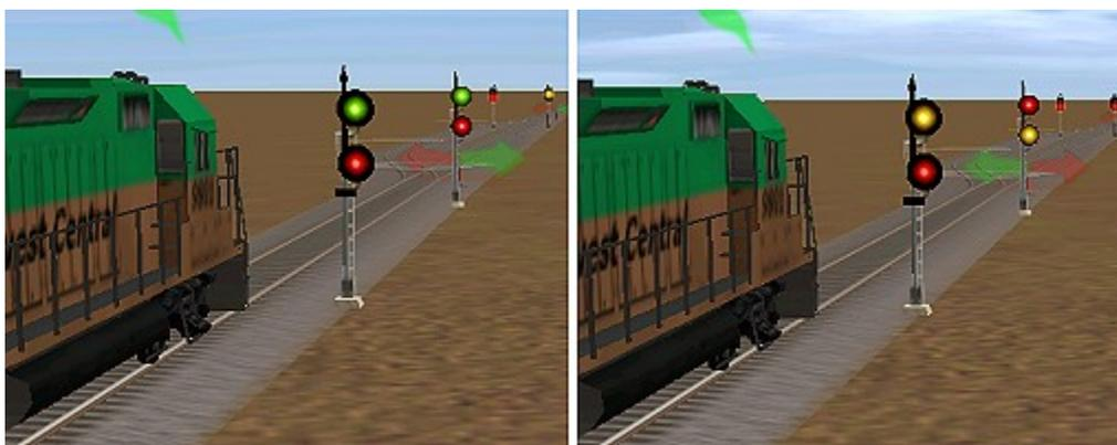
In the pictures above, we have an '03' signal just in front of the loco. The next signal is a 'L02' (since the junction diverges left) and there are '04's' down at the end of the pass track. (Hmm. Looks like I used 'USA 2 04's' instead of regular '04's' down there, but that's okay, they work the same way.)
