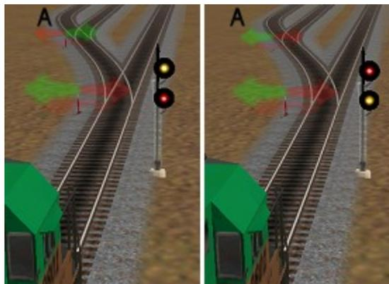
In the drawings above, we have a small industry area branching off the mainline. With the mainline switch aligned toward the industry, you would expect to see a red-over-yellow (or perhaps red-over-green) signal, indicating the divergence. Instead, in the left picture, we see yellow-over-red, which appears to be a normal mainline caution signal.
