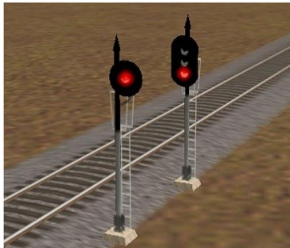
These signals are USA-04, on the left, and USA 2-04. (In Surveyor, they are called 'Signal USA 04' and 'Signal USA 2 04'). These signals can display all three aspects, with the USA 04 changing colors as necessary.
