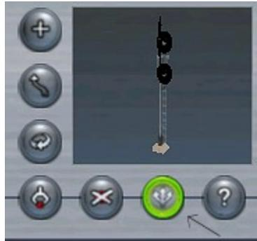
With the tool selected, click on the turnout you want to test. You should see the green/red switch indicator change from one side to the other, an indication the switch is working. If there's a signal associated with the turnout, you'll see the signal change as well.
