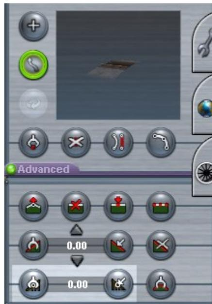
The highlighted portion at the bottom of the picture above shows the vertex height tools. Selecting the left button and clicking on a spline gets the height of that spline and places it in the display window. Selecting the right hand tool allows you to assign the track height displayed in the window to one or more other splines.
